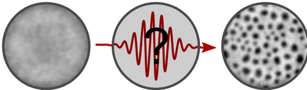
FIG: Schematic illustration of skyrmion nucleation. The talk will focus on the mechanism and speed of how such skyrmion nucleation can be induced by spin-orbit torque current pulses and femtosecond laser pulses.
